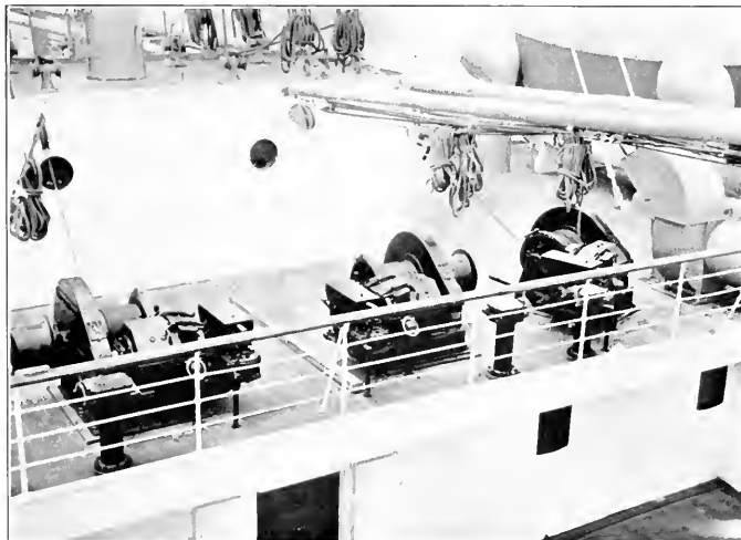
View of the top of the house at the after end of bridge deck showing three of the four cargo winches serving the after cargo hatch. Note power substation erection at the base of the mast for housing control apparatus for winch motors.
